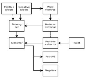
Fig. 2.architecture diagram sentiment analysis
